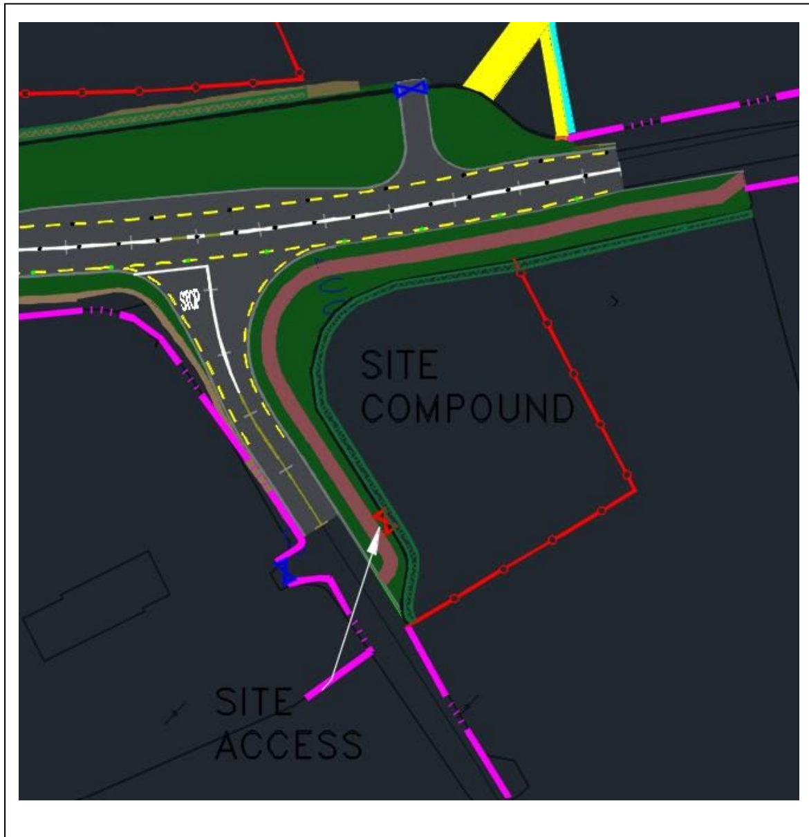
Figure 2.5: Proposed Site Compound & Access
